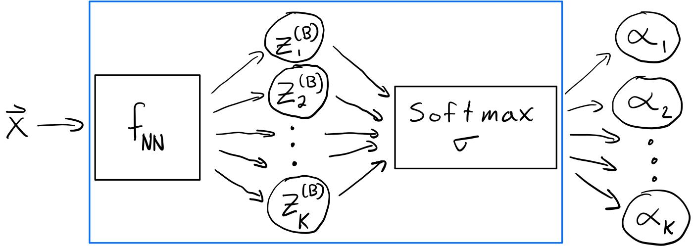
$$f_{\text{prob}}(\vec{x}) = \sigma(f_{\text{NN}}(\vec{x})) \in \mathcal{Y}_{\text{prob}}$$
